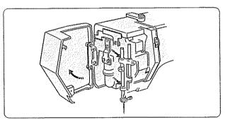
Open tace cover plate and oil points as shown below at least once a year. One or two drops of oil is sufficient.
